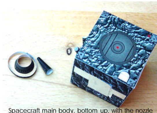
Spacecraft main body, bottom up, with the nozzle of the main engine, the separation ring and the nozzle protection on the left
