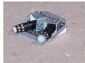
Star tracker mounted on the platform
